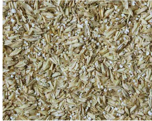
Figure 1. Grind profile from a 4-roller Mill consisting of very coarse, non-uniform crumbs of slightly cracked and crushed kernels.
