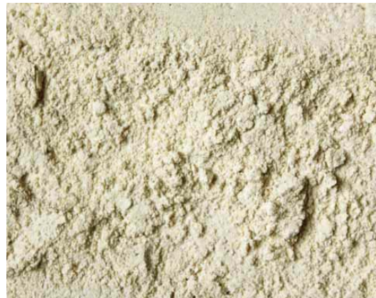
Figure 2. Grind profile from a Fine Grind Mill consisting of extremely uniform particles, ranging in size from 100 - 10 microns.
